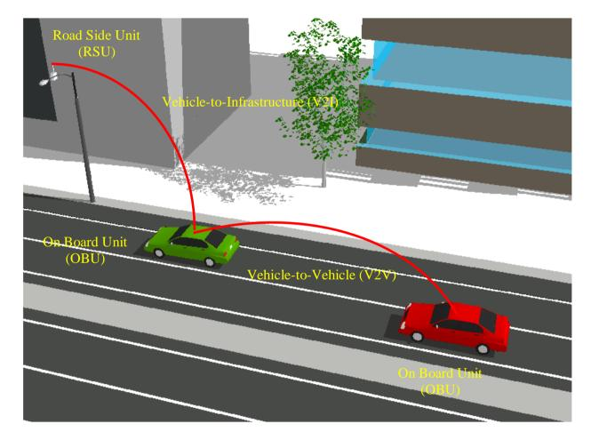
Vehicles on the road will constantly be transmitting data such as their position, speed, and heading. This will allow other vehicles to determine if a collision is likely and to take appropriate action. For example: imagine two vehicles approaching a blind intersection. By analyzing the transmissions from the other vehicle, a vehicle can determine if a collision is likely and warn the driver.
