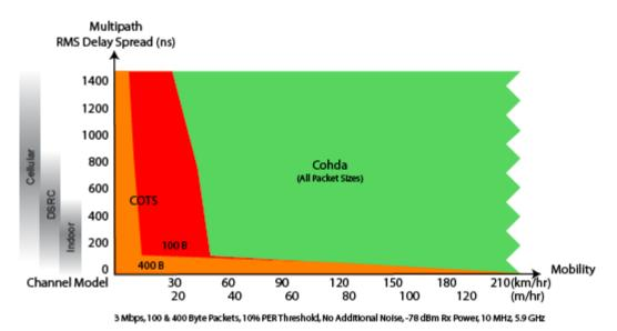
In addition to being robust under conditions of simultaneous multipath and mobility, Cohda's DSRC radios also have improved receiver sensitivity and increased tolerance to interference.
