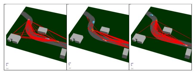
Now, how does this multipath and mobility affect a DSRC radio in practice? In the following plot we show the results of bench tests of a typical commercial off-the-shelf (COTS) DSRC radio using a channel simulator. Channel models with differing RMS Delay Spreads – a measure of multipath – were tested at a variety of different vehicle speeds.
